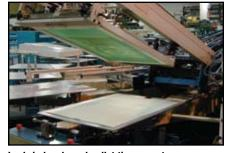
Lock-in heads and pallet tip supports ensure even tone coverage from front to back. Ideal for four-color work.
