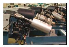
Electro-mechanical drive systems provide smooth print/flood stroke regardless of image size.
