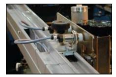
Stroke length sensors work anywhere within the print area by adjustable slides.
