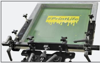
Sturdy side screen clamps ensure stability, improving production quality and efficiency.
