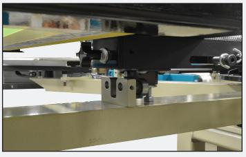
Heavy-duty lock-in print head facilitates precise multicolor printing.
