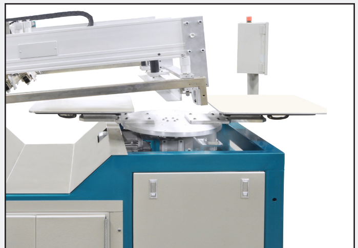
Side view shows motor-driven indexer and easy access to screens and press setup.
