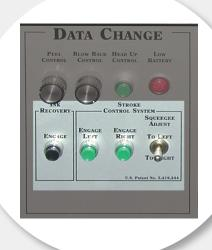
The Automatic Computer-controlled Stroke Setting allows the operator to set stroke from up-front control panel without moving sensors.
