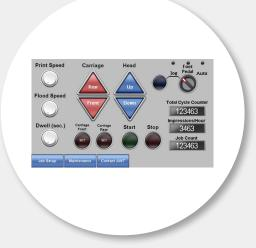
The touchscreen allows the operator to control a variety of functions such as print and flood speeds, carriage and print head position and cycle counts, with a simple touch.
