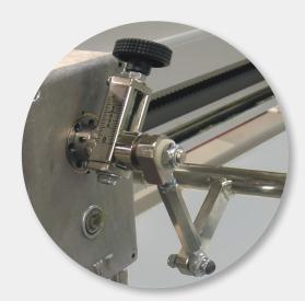
Exclusive upfront peel system gives operator quick and convenient control of peel rate setting.
